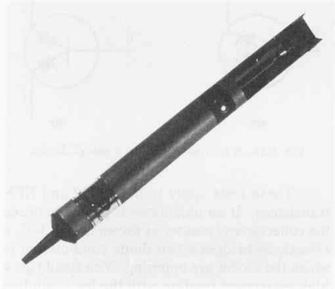
Fig. 3-27. The spring-driven plunger in the solder vacuum pump is used to pull hot solder off a connection.
