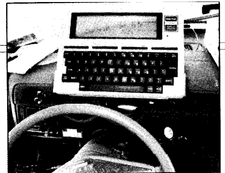
Photo 1. My Model 100 computer, mounted on the dash of my motor home, with the Car Navigator program running.
