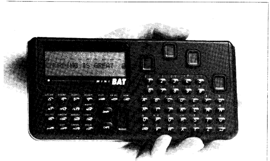
The MiniBAT uses a unique set of five buttons to allow keyboard touch typing with one hand.
