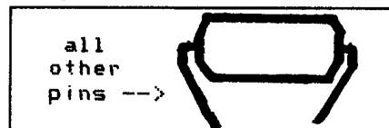
Figure 3. An end view of the RAM chip, showing all the pins except 20 and 22 are bent in toward the body of the chip.
